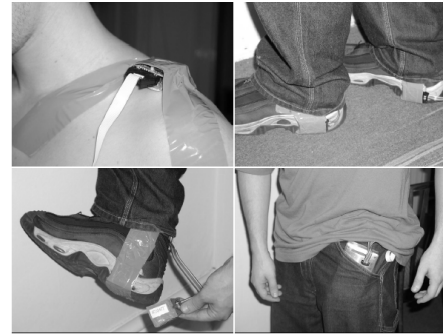
Figure 7. Clockwise from top left: compass sensor taped to shoulder; accelerometer sensors attached to pedestrian's shoes; Bitsy motherboard carried in pocket; and accelerometer sensor, extracted from sole holster to show size.
