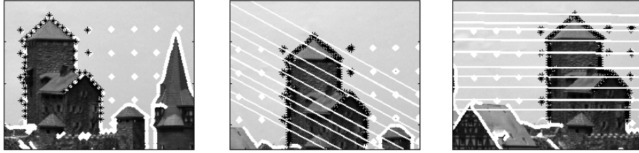
Figure 4: Three images from the Castle sequence, and some of the epipolar lines.
