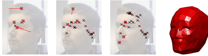
Figure 3: The sample matches (red squares) used to calculate a motion hypothesis and the other matches (black crosses) which support the hypothesis. The likelihood of the pose increases from left to right, the model showing the final pose hypothesis.
