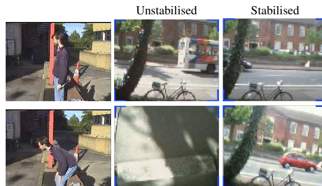
Fig. 4. Samples from a sequence obtained while the wearer sits down in an outdoor scene.
