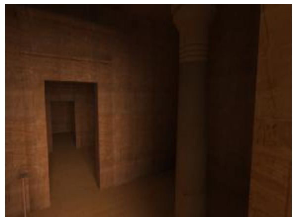
Figure 5: The first room rendered with using mkillum and with changed parameters (ab=2)
