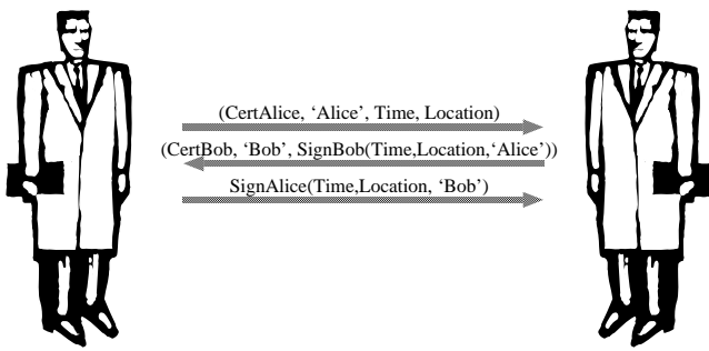
Figure 2. Protocol for obtaining an authentic record of the time and location of a meeting
