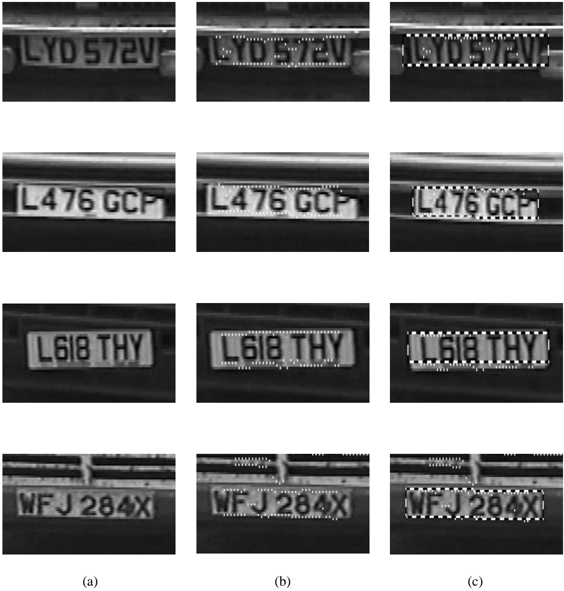
Figure 4.10: Several possible plates (a), the estimates for their tops and bottoms (b) and the best fits of the number-plate model (c)
