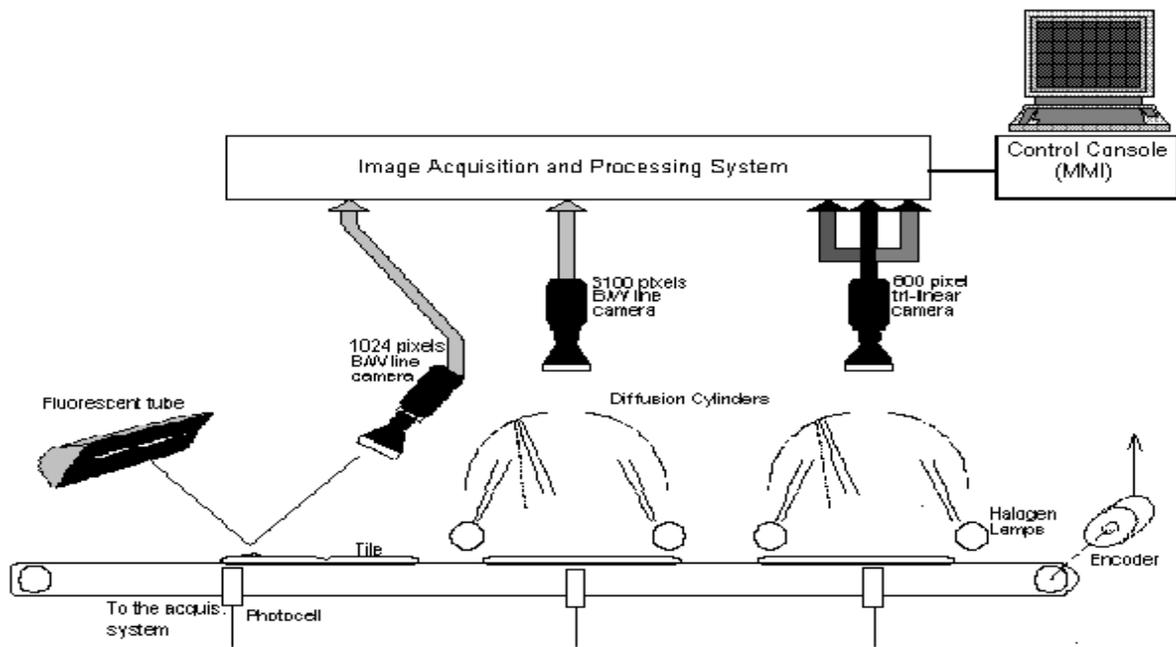
Figure 1: Overall ASSIST system structure
